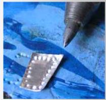
Use a pointed object to press the rivets into the material (Use some kind of piece of wood underneath to protect the dining table or your mother/girlfriend/wife will most definitely explode!) Then it is a simple matter of gluing the plate in place where you want it.
